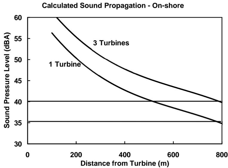
Figure 1: Predicted Sound Pressure Level vs. Distance from Turbine
