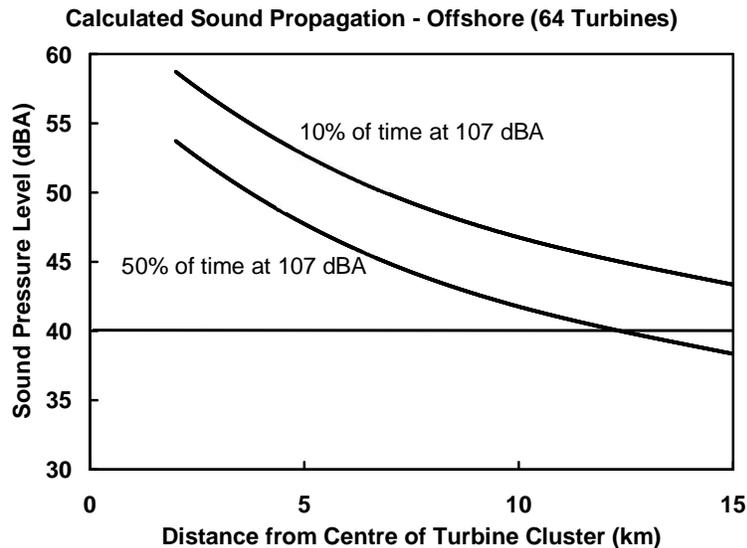
Figure 2: Predicted Sound Pressure Level vs. Distance from Group of 64 Offshore Turbines
